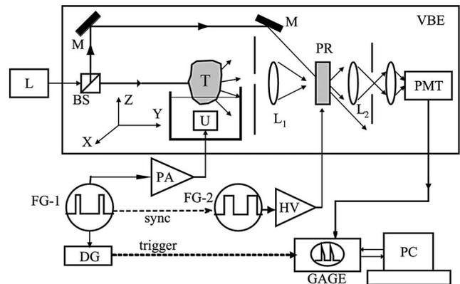
Fig. 1. Schematic of the experiment setup: L, laser; BS, beam splitter; M, mirror;  $L_1$ ,  $L_2$ , lens; PR, photorefractive crystal BSO; PMT, photomultiplier; FG-1, FG-2, function generators; PA, power amplifier; DG, pulse-delay generator; HV, high voltage amplifier; PC, personal computer; U, 1 MHz ultrasound transducer; T, study sample; VBE, vibration block enclosure; GAGE, CompuScope 14200 14 bit waveform digitizer.
