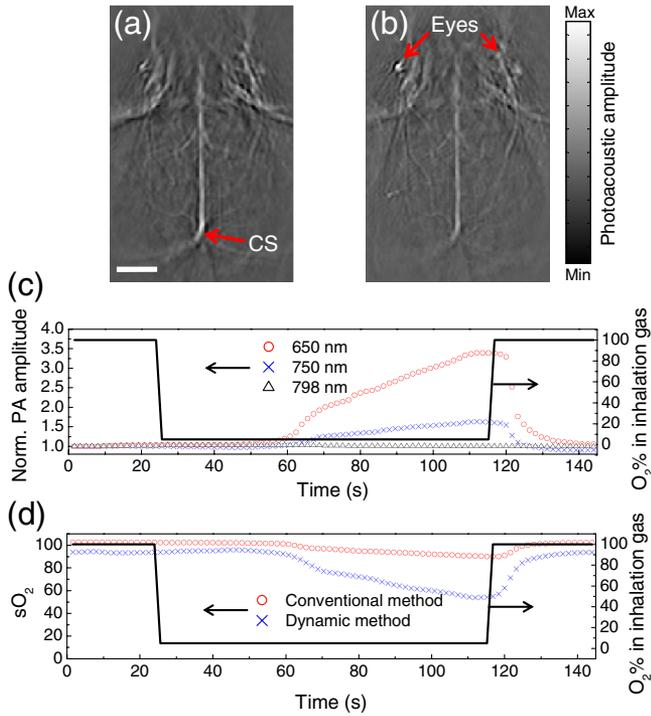
Fig. 4. *In vivo* experimental results. Photoacoustic images of cortex vasculature acquired noninvasively at (a) 650 nm and (b) 750 nm laser wavelengths. Scale bar: 2 mm. (c) Changes in photoacoustic amplitude at different wavelengths in the superior sagittal sinus. (d)  $sO_2$  calculated based on the conventional and the new dynamic methods. (Media 3, QuickTime, 7.6 MB).
