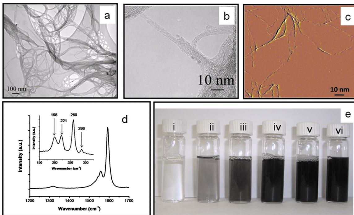
**Fig. 1** (a) A low-resolution bright-field TEM, (b) HRTEM image of bundled SWNTs grown using Fe as the catalyst. (c) Tapping mode AFM images of dispersed SWNTs. (d) D-band and G-band Raman spectra of the SWNTs. The inset shows the radial breathing modes. (e) Vials contain aqueous dispersions of SWNTs in Pluronic F127 after being sonicated. From left to right, the concentrations are (i) 0, (ii) 0.1, (iii) 0.25, (iv) 0.5, (v) 0.75, and (vi) 1 mg/mL. (Color online only.)
