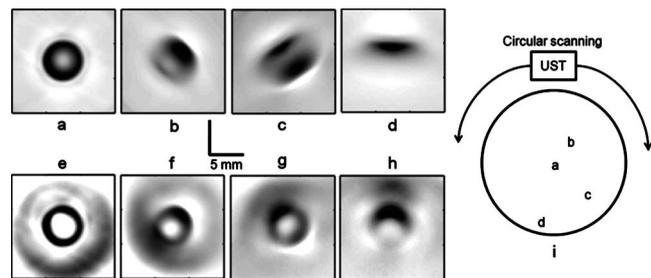
**Fig. 5** Reconstructed cross-sectional TAT images, using the flat ultrasonic detector, of an LDPE tube (~1 cc volume; inner diameter ~6 mm) filled with salt water placed at distances of (a) ~2 mm, (b) ~23 mm, (c) ~39 mm, and (d) ~49 mm from the scanning center, respectively. Corresponding TAT images obtained with the negative lens detector are shown in (e), (f), (g), and (h), respectively. (i) Location of the tube inside the scanner is shown.
