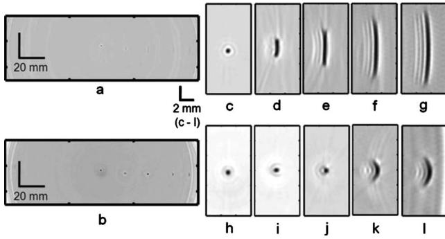
**Fig. 3** PAT images of five 0.5-mm-diam pencil leads placed inside the scanning region at different distances from the scanning center. (a) Reconstructed PAT image using the flat detector. (b) Reconstructed PAT image using the negative lens detector. (c) to (g) Close-up images of all five objects in (a) at distances of ~2 mm, ~19 mm, ~36 mm, ~55 mm, and ~67 mm from the scanning center, respectively. (h) to (l) Corresponding close-up images obtained with the negative lens detector.
