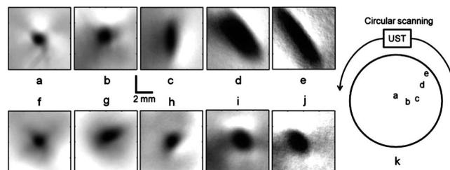
**Fig. 2** Reconstructed TAT images, using the flat ultrasonic detector, of a needle (18 gauge, 1 mm in diameter) inserted inside a pork fat base placed at a distance of (a)  $\sim 4$  mm, (b)  $\sim 14$  mm, (c)  $\sim 32$  mm, (d)  $\sim 50$  mm, and (e)  $\sim 64$  mm from the scanning center. Corresponding TAT images obtained with the negative lens detector are shown in (f), (g), (h), (i), and (j), respectively. (k) Location of the needle inside the scanner is shown.
