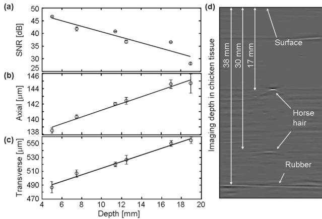
**Fig. 2** (a) SNR versus imaging depth (depth of the ultrasonic focal point). (b) Axial resolution versus imaging depth. (c) Transverse resolution versus imaging depth. (d) Demonstration of the maximum imaging depth ( $\sim 38$  mm) in chicken breast tissue.
