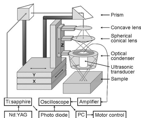
**Fig. 1** Schematic of the deep reflection-mode photoacoustic imaging system.
