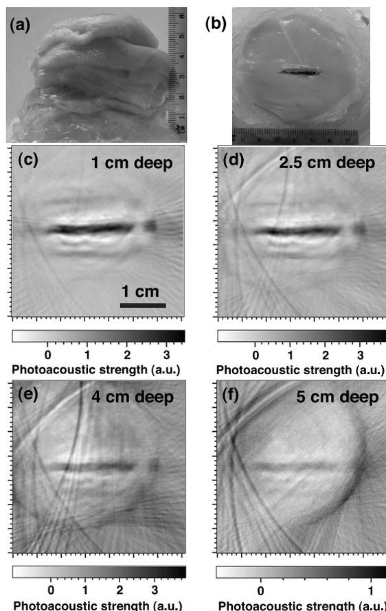
**Figure 5:** Two-dimensional photoacoustic images of a blood object in chicken breast muscle. Photograph of (a) the entire test sample and (b) the blood object embedded in a cross section of chicken breast muscle. Two-dimensional photoacoustic images acquired with a 3.5-MHz ultrasonic transducer at depths of (c) 1 cm, (d) 2.5 cm, (e) 4 cm, and (f) 5 cm, respectively, in chicken breast muscle.
