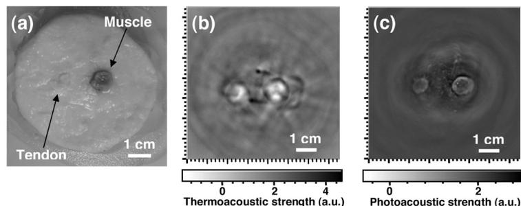
**Figure 3:** Thermoacoustic and photoacoustic images of porcine muscle and tendon in fat tissue. (a) Photograph of the tissue sample. (b) Thermoacoustic image. A U-shaped metal wire placed on the tissue sample was imaged along with the muscle and tendon. (c) Photoacoustic image.
