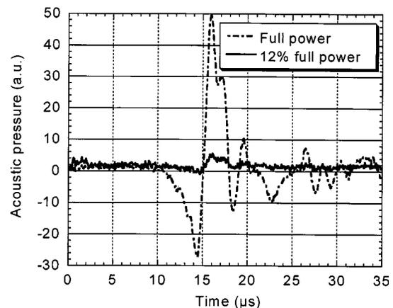
FIG. 3. Waveforms of the microwave-induced acoustic pressure when the sample was exposed to the full power of the microwave generator (0.55 mJ/cm<sup>2</sup>) and to 12% of the full power.
