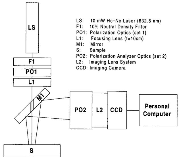
Fig. 3. Schematic diagram of the experimental setup.
