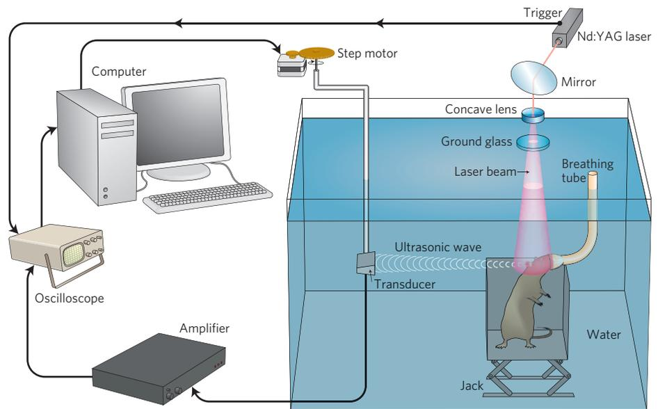
**Figure 1** | Schematic of a photoacoustic system for imaging the brain of small animals. Systems can also be equipped with a microscope to allow imaging of smaller target areas. The sample is immersed in water to allow high-quality collection of the ultrasonic acoustic waves. Adapted from ref. 1. © 2003 NPG.
